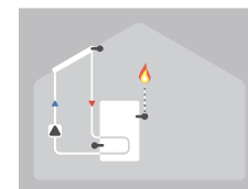
Solar with thermostat (auxiliary heating)
