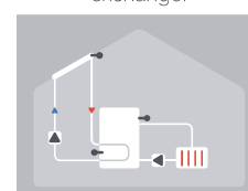
Solar with cooling 3 (panel cooling)
